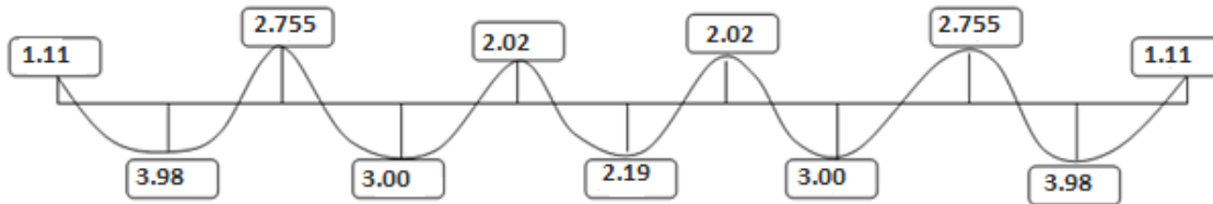
Figure (III.11) : diagramme des moments a ELS.
