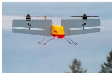
Aile inclinable Tilt-rotor and tilt-wing
