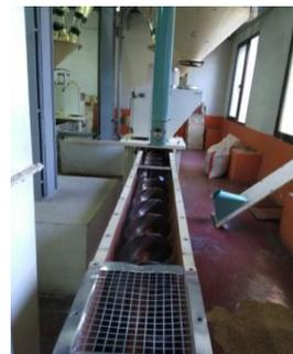
Figure 57 : Vis collectrice (original)
