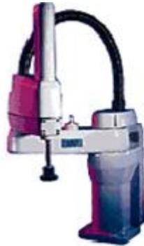
Figure 1.6 : Robot SCARA. [5]
