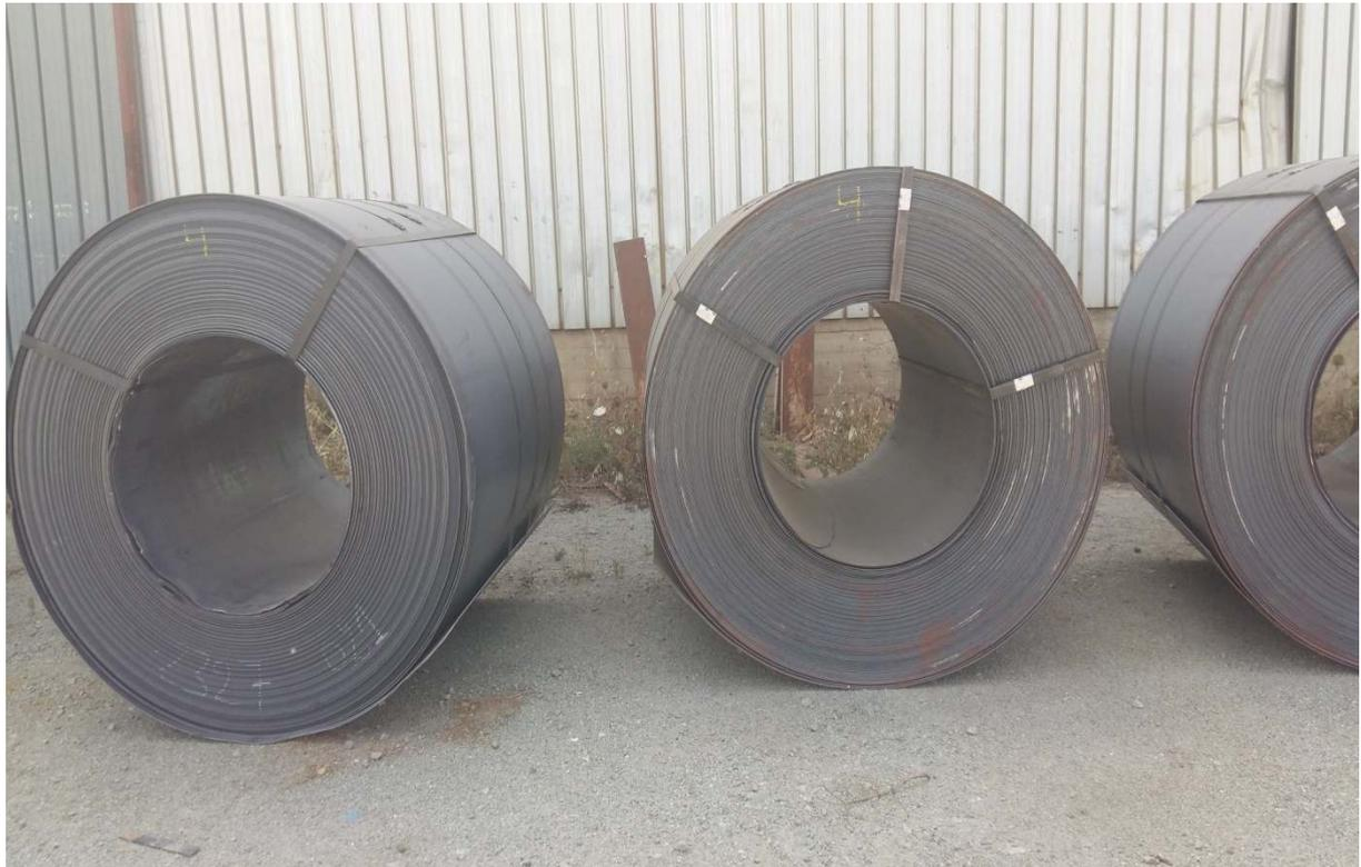
**Figure I-2:** Bobins d'acier S235JR.
