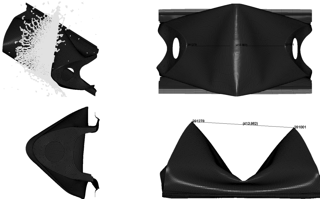
Figure 4.21. 8 lb bird striking onto Al 6013 T6 Alloy LE bay with a velocity of 129 m/s
