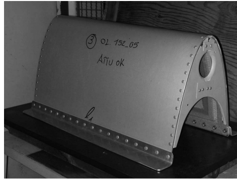
Figure.3.23. View the leading edge bay [30]
