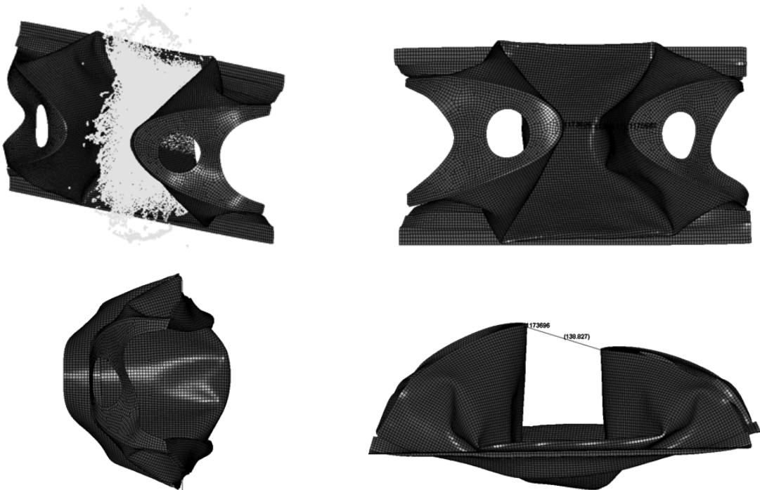
Figure 4.24. 8lb bird striking onto composite FML LE with a velocity of 129 m/s
