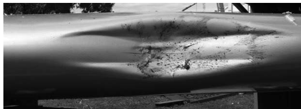
Figure.3.33. Ribless sandwich FML LE after impact of 8 lb bird at 129 m/s, Exp [82]
