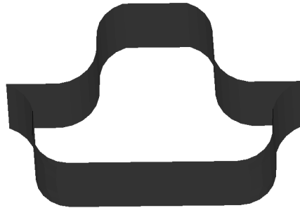
Figure 4.18. Unit cell of F40- 0.0019- 5052- 3.1 pcf honeycomb
