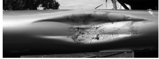
Figure 4.34. Front views of the ribless sandwich FML LE after 4 lb and 8 lb bird impacts at 129 m/s ( the 8lb bird impact test on the S.FML. LE has been already validated in Chapter 3)
