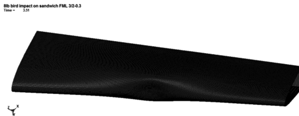
Figure.3.31. Final shape of the ribless sandwich FML LE after the 8 lb bird impact at 129 m/s
