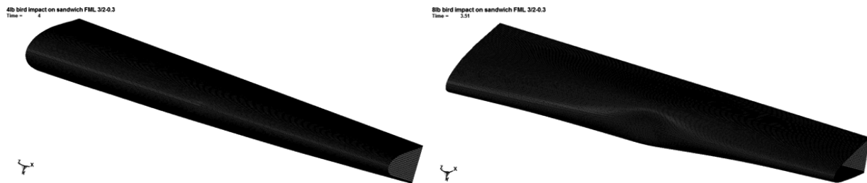
Figure 4.33. 3D views of the ribless sandwich FML LE after 4 lb and 8 lb bird impacts at 129 m/s
