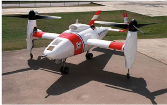
Figure 1.2: The Eagle Eye is a tilt-rotor UAV
