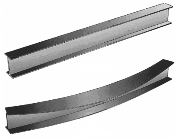
Figure 6.2: Lateral buckling phenomena
