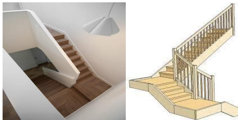
Figure 1.8: Half turn stair.
