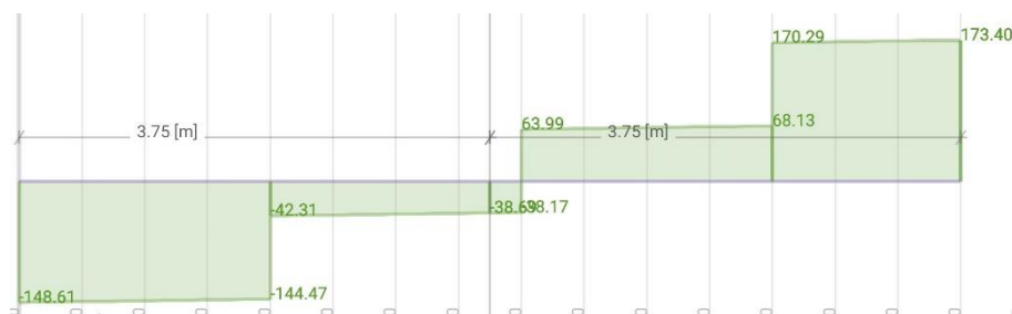
Figure 3. 10: shear force diagram for the main beam. (Final phase)
