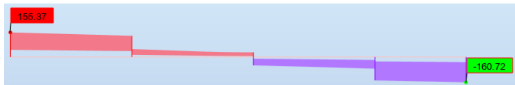
Figure 5. 2: Shear force diagram for the main beam.
