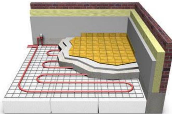
*Figure 1.08 Plancher chauffant*
