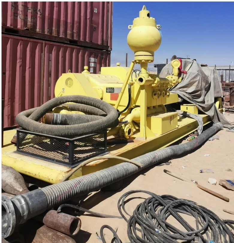
Figure 11 : Pompe a boue triplex simple effet.
