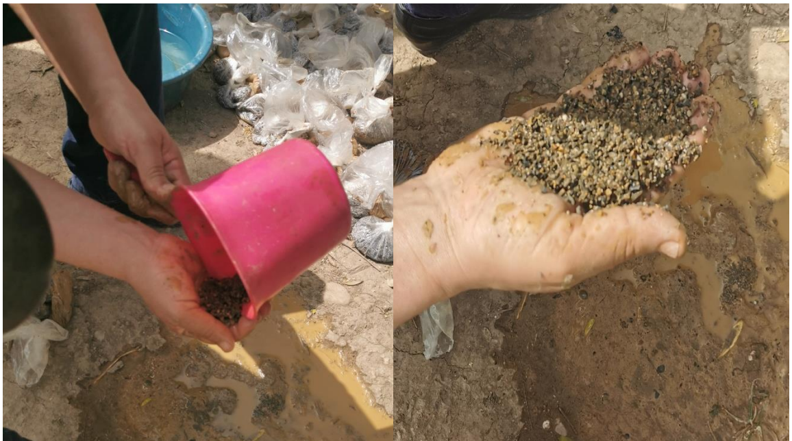
Figure 29 : lavage des cuttings.
