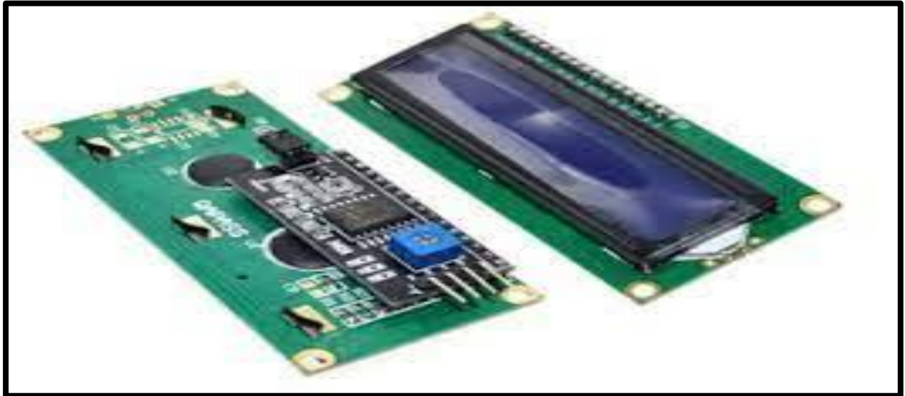
Figure 2.24: Afficheur LCD et I2C
