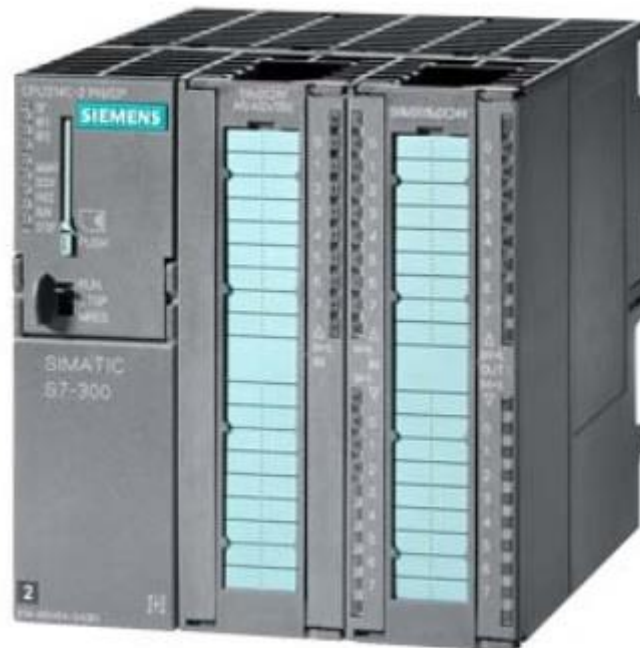
Figure 2.22 :CPU Siemens SIMATIC S7 314C-2 PN/DP [40].
