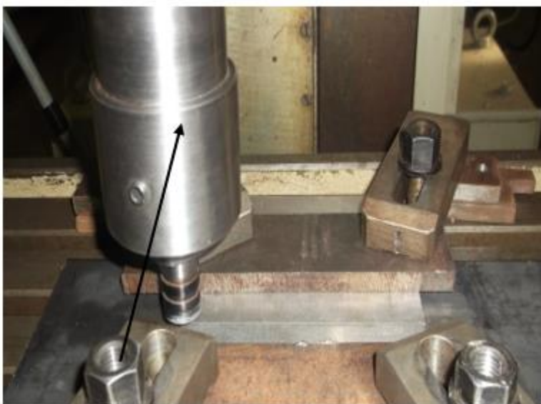
Figure II.16 — Outil du soudage FSW
