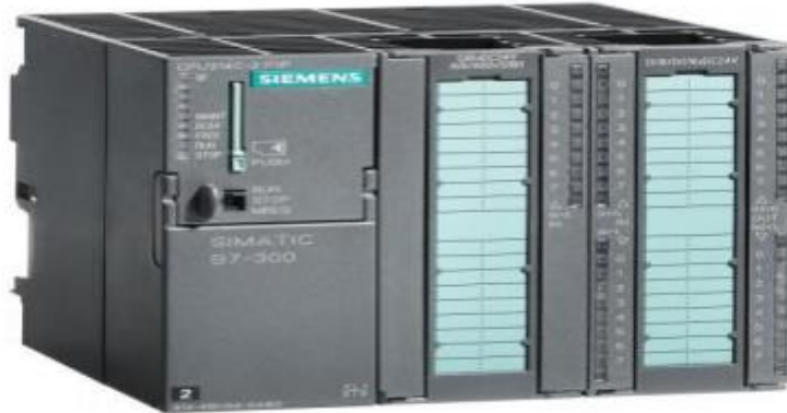
FIGURE 2.6: Automate SIEMENS S7-300.
