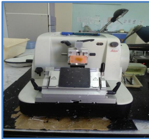
Figure 29: Microtome de type Leica (Photo personnel)
