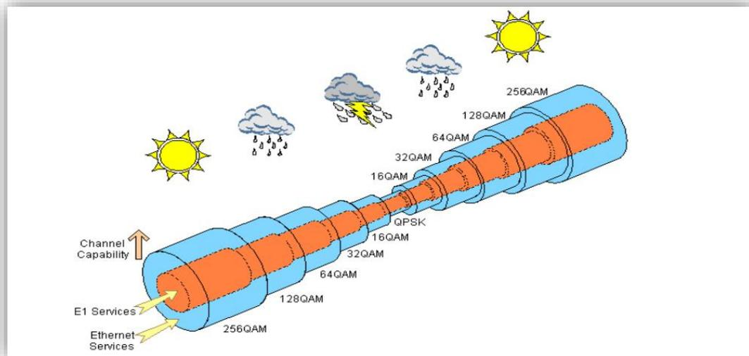
*Figure 2. 9:* Modulation Adaptative.
