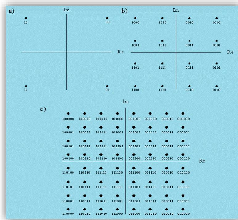
Figure 1.15: Modulation QAM.
