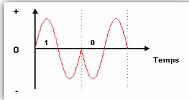
*Figure 1.11: Modulation PSK.*
