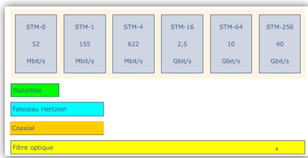
Figure 1. 23: Les supports de la SDH.
