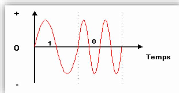
*Figure 1. 14: Modulation FSK.*
