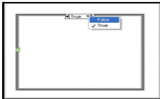
Figure (3.6) Case structure.
