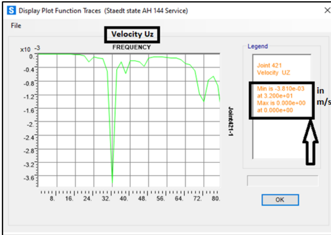
Figure III-14 The velocity diagram on the joint 421
