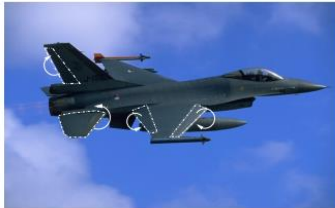
Figure 2.7: Control Surfaces of an F-16 Model [7].
