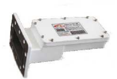
Figure IV.4 : Le LNB. (Low Noise Block)
