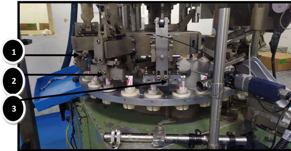
Figure II.9 : Station de fermeture
