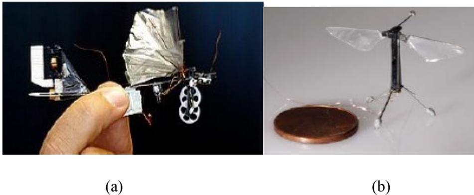
**Figure I-13 :** (a) Le micro Delfly,(b) Le Robobee
