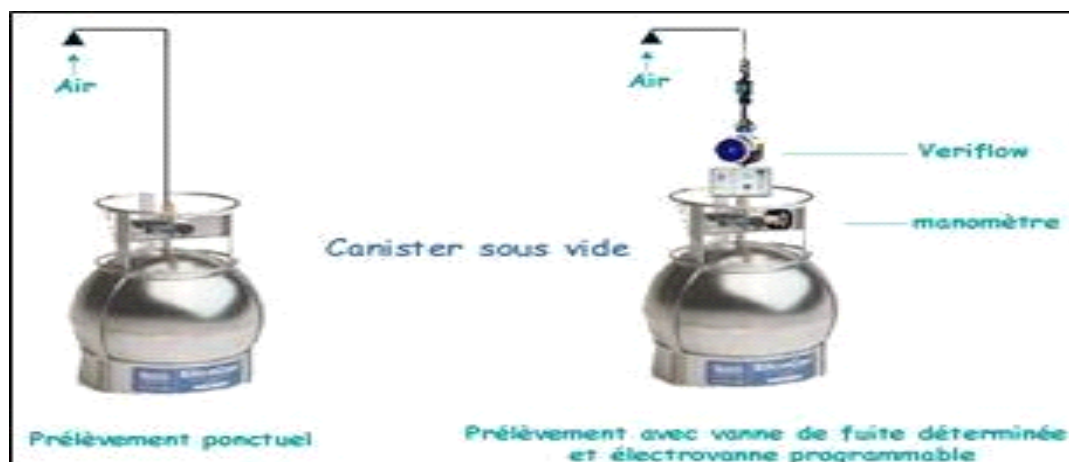
Figure N°20: Principe du canister (ASQAB, 2007)
