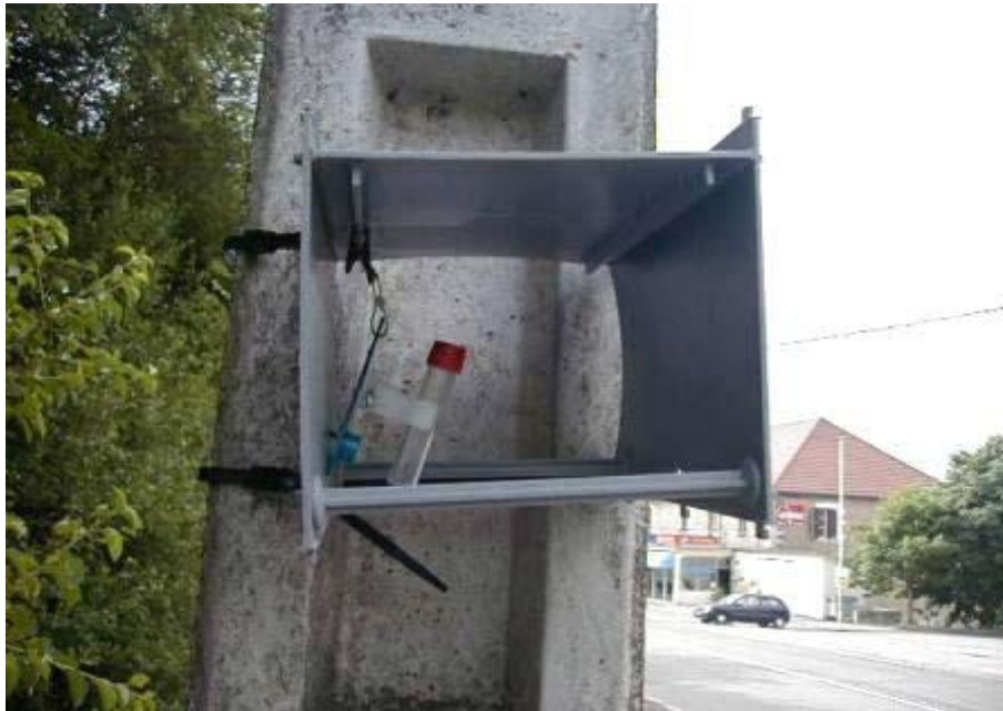
Figure N°6 : Échantillonneur passif (ASQAB, 2007)
