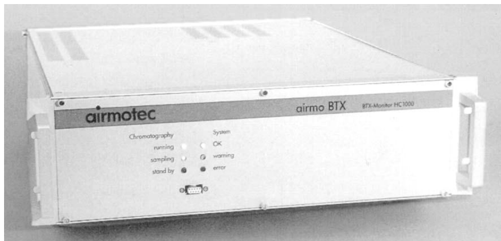
Figure N°22 : Analyseur de BTEX GC on-line Airmo BTX de Airmotec (Badjagbo.K, 2009)
