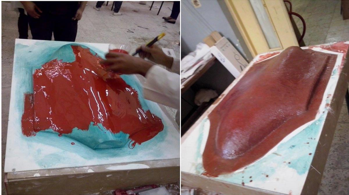
**Figure (IV-17) :** Application de gelcoat.
