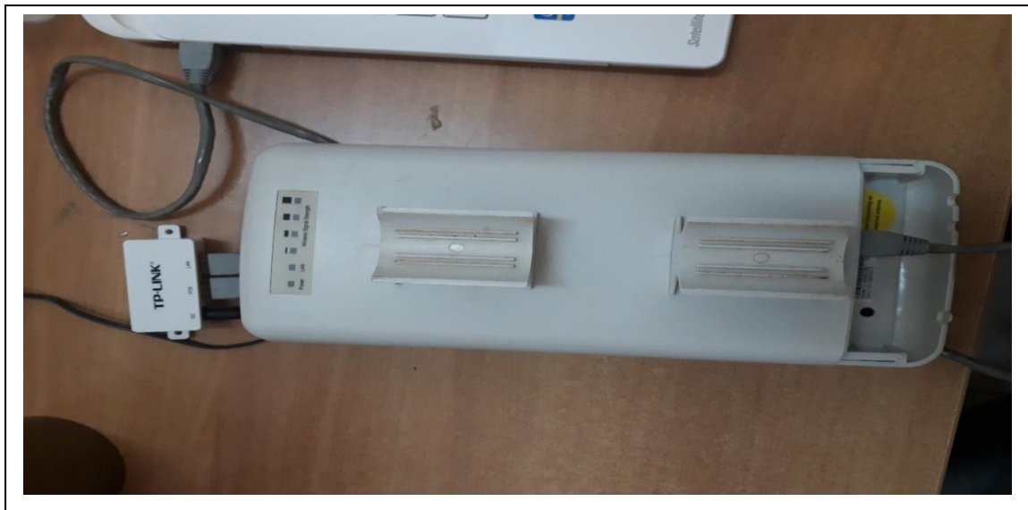
Figure III.4: Branchement de l'antenne TP-LINK-TL-WA5210G
