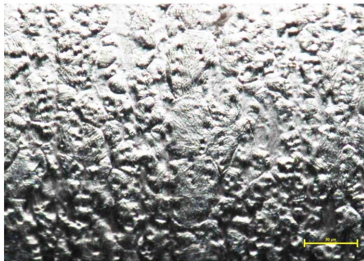
Figure 15: microstructure trempe z160 *200
