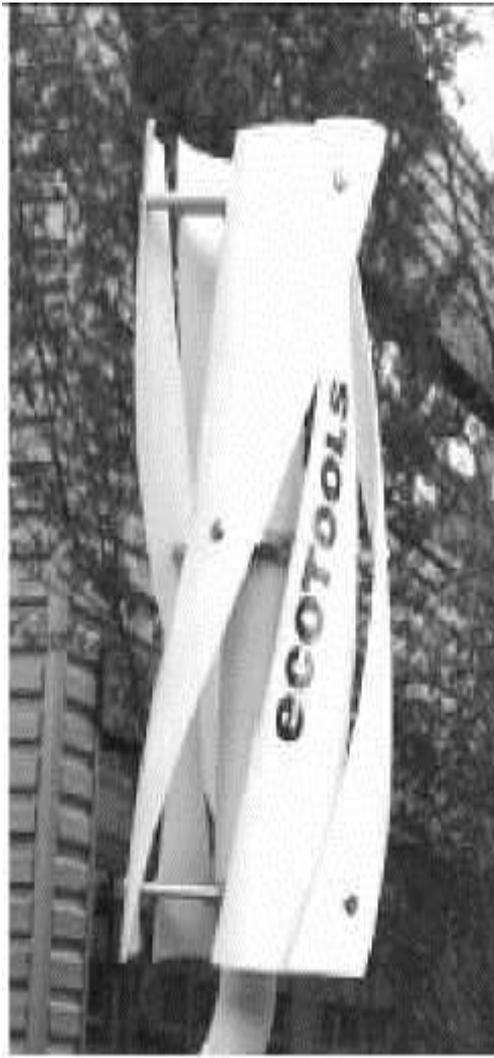
Figure I -14: Turbine Savonius
