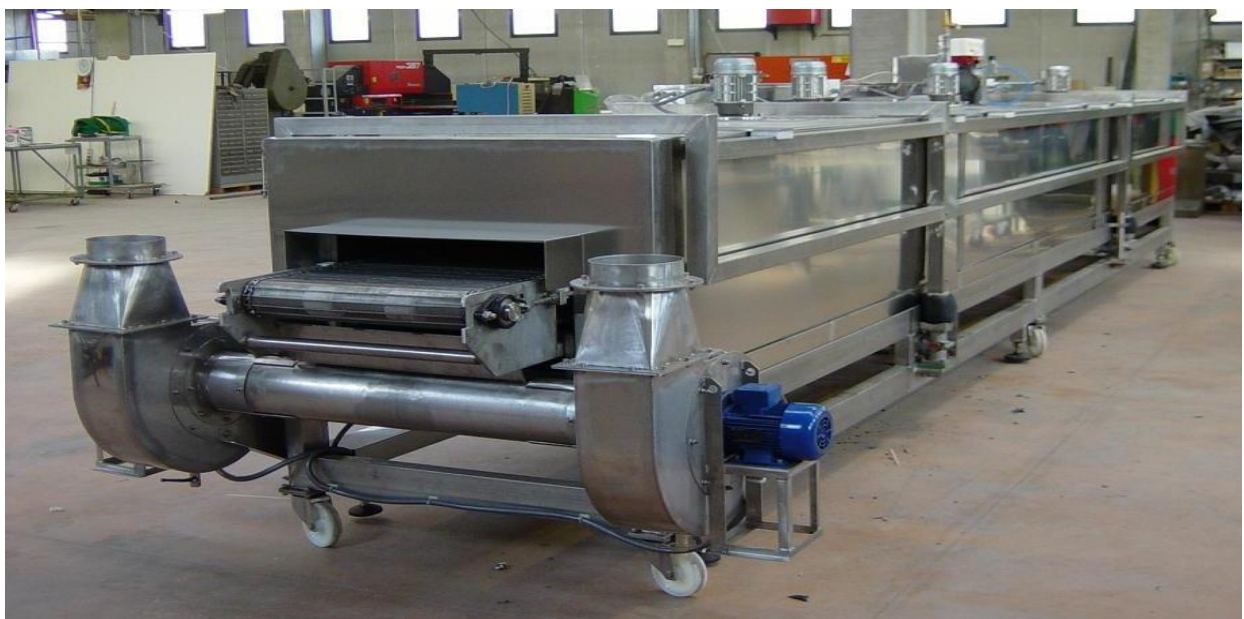
Figure (1.6) : Tunnel de congélation.
