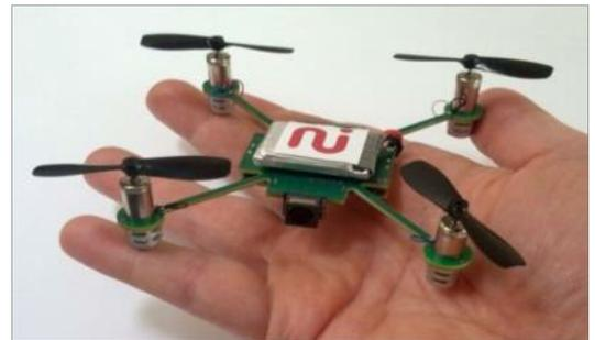
Figure I-13 : Micro-drone quadri rotor.
