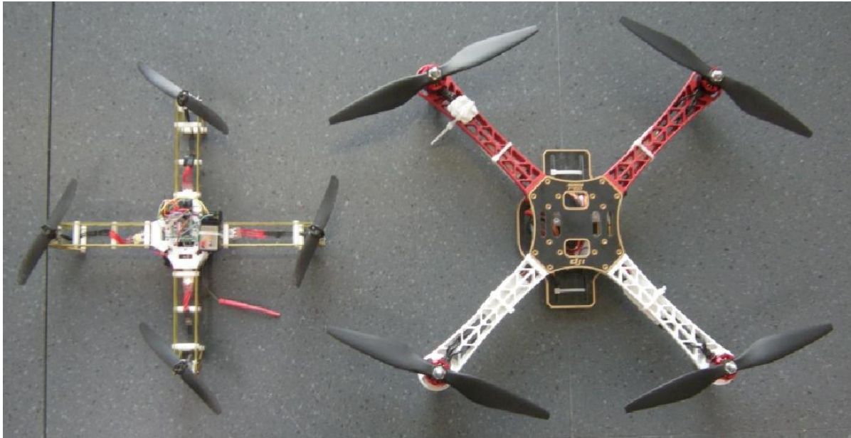
Figure II.2: Quad "+" et Quad "X"
