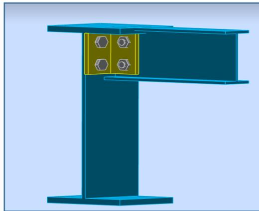
Figure 7.4 : Assemblage poutre IPE 400 – solive IPE 120.
