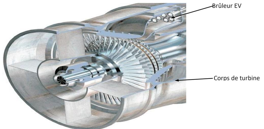
Figure 3-7 : section turbine
