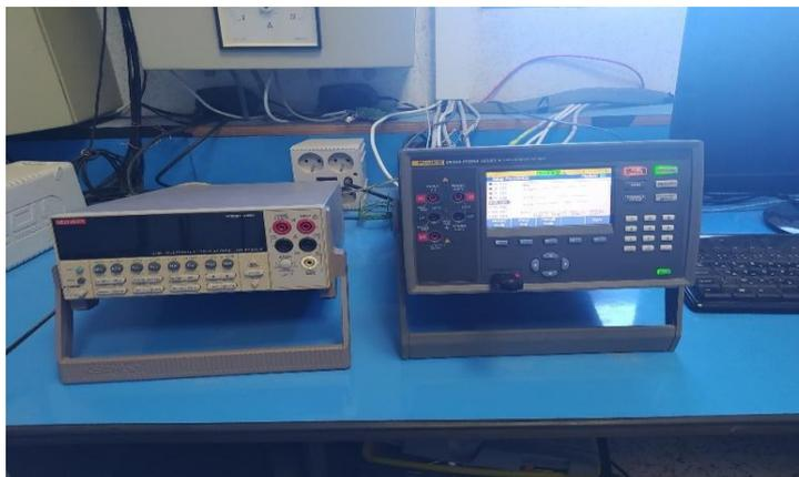
Figure IV.2 : FLUKE 2638A Hydra series III data acquisition
