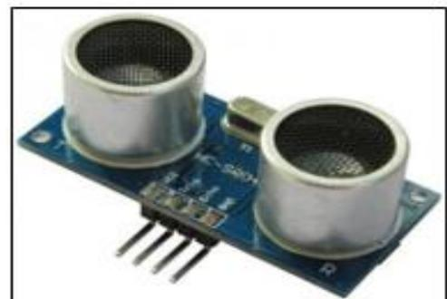
Figure III-6 : Ultrason HC-SR04.
