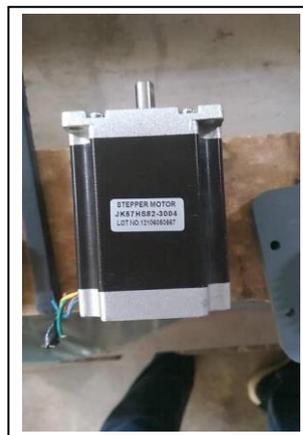
**Figure IV.3: STEPPER MOTOR JK57HS82-3004**
