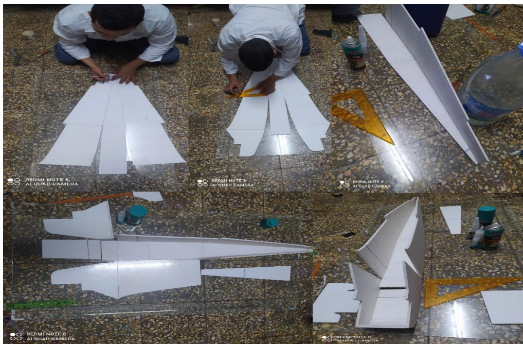
Figure IV-25 Collage les pieces de fuselage.
