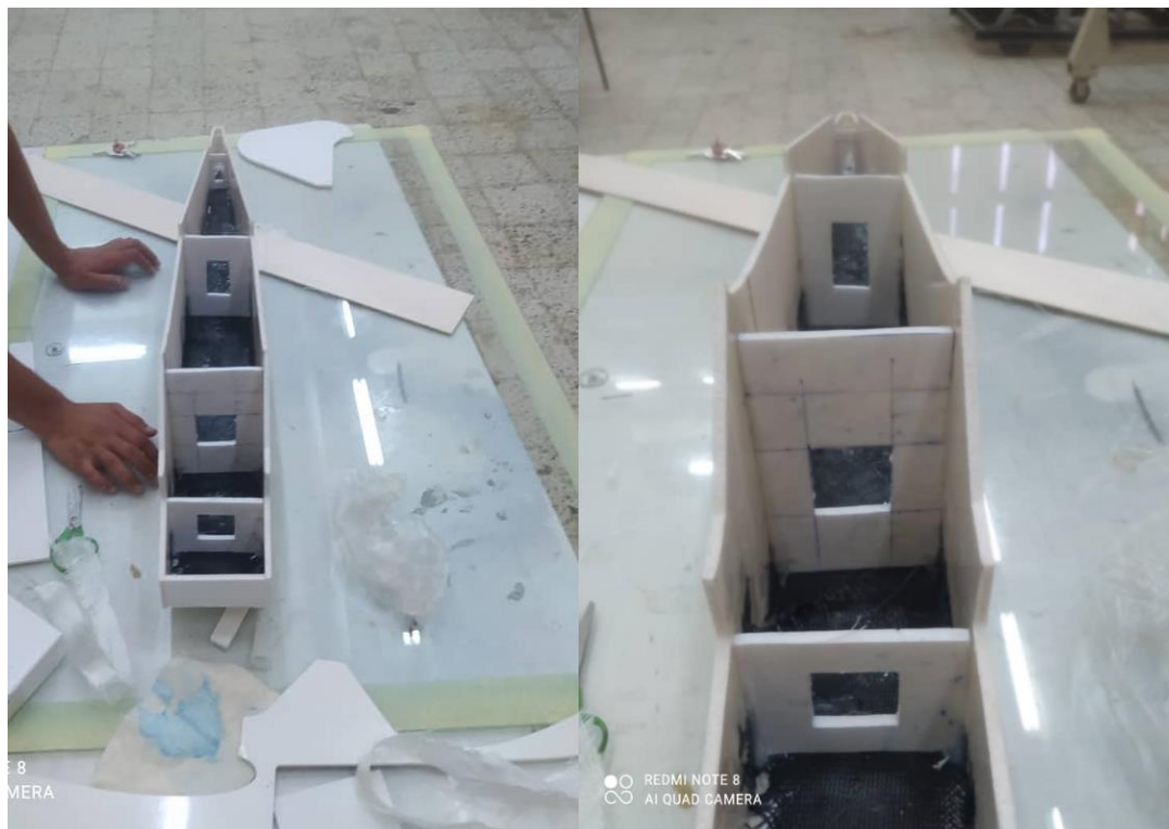
Figure IV-27 Renforcement les differentes stations de fuselage.
