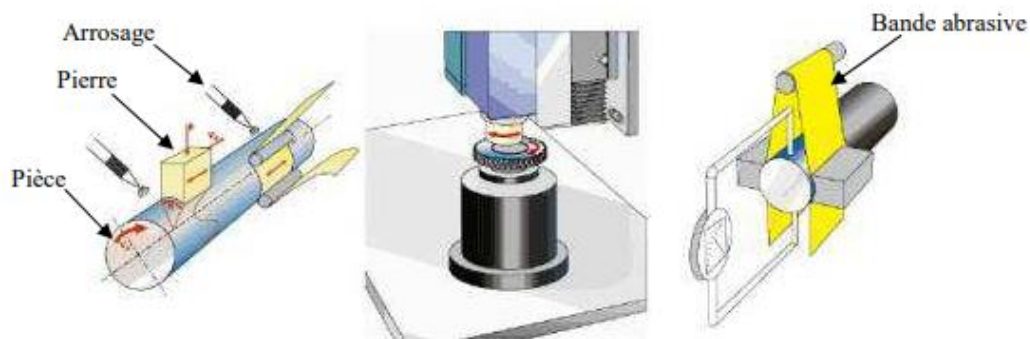
Figure II.19 : Principe de la super finition.
