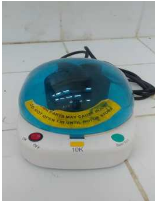
Figure IV.6. Centrifugation of isopropyl and Bismuthene mixtures
