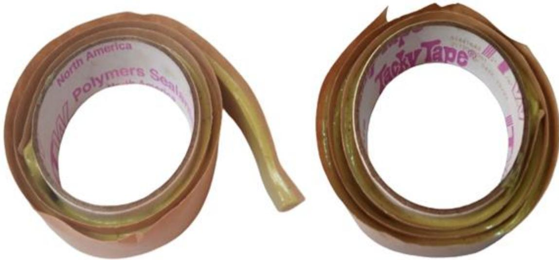
Figure 2.11 : Vaccum bag Sealant, tape coulant [3].
