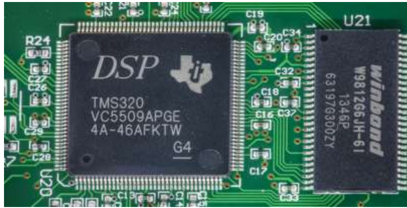
Figure 1.2 Le Digital Signal Processor DSP. [4]
