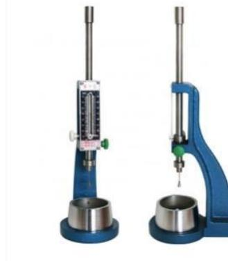
**Figure III.11 :** Appareil de Vicat manuel.
