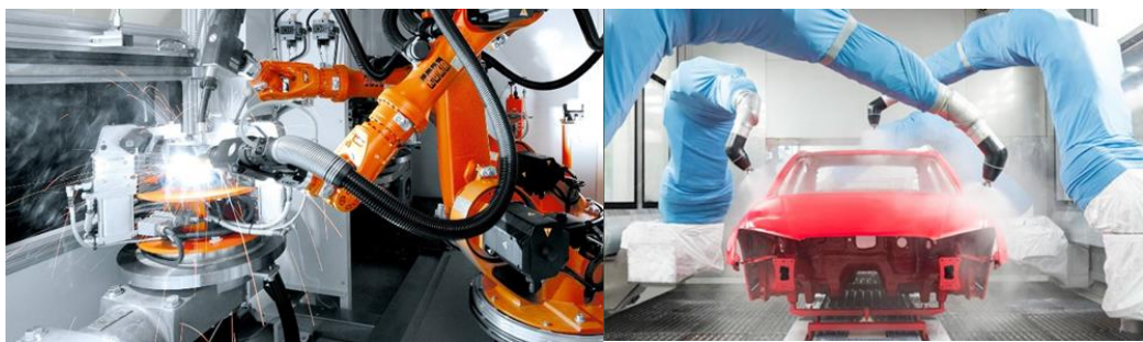
Figure 2-1: Robot arms during spot welding and surface.
