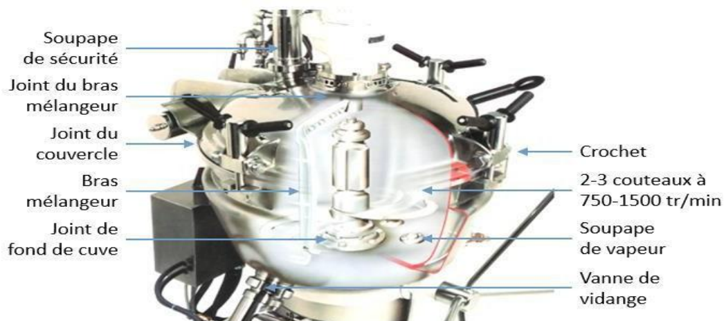
Figure 1.9: Composant d'une cuve cutter [4]
