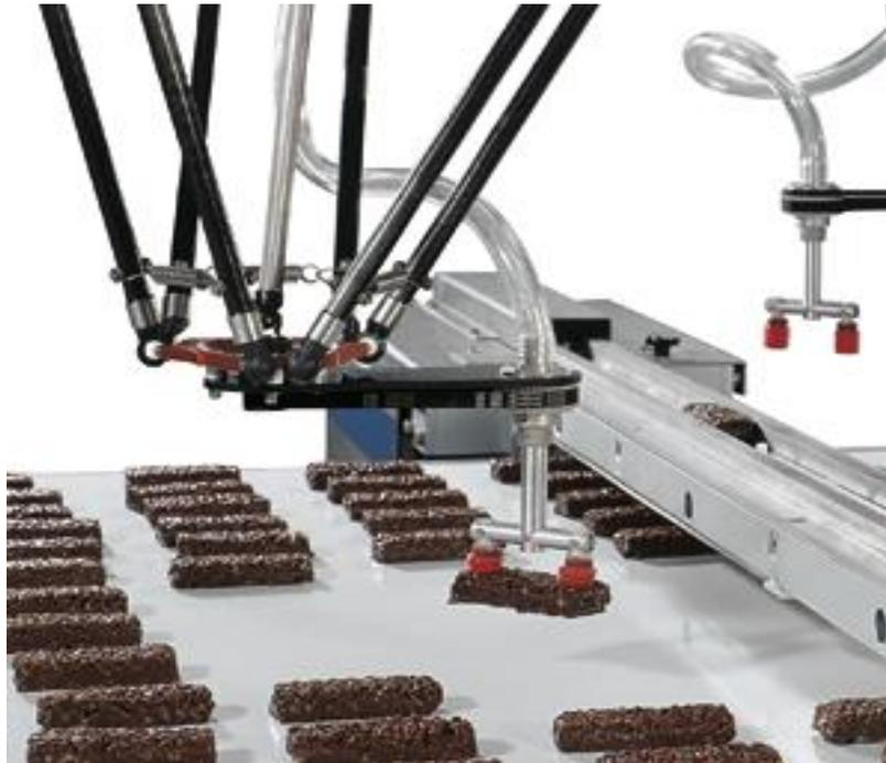
Figure 1.4 – Robot Parallèle (Pick & place)
