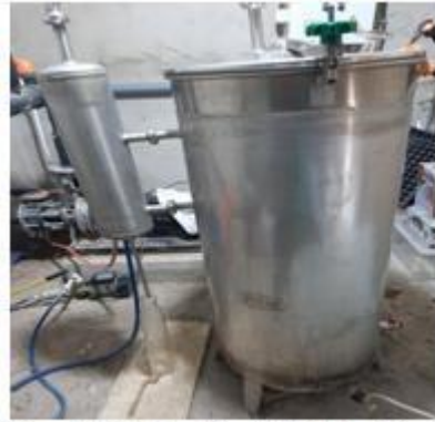
Figure (II.4) : Alambic de 200 L (original, 2021)
