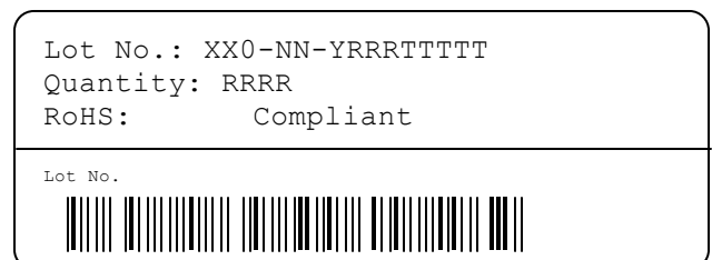
Figure 14: First label on reel: XX = Sensor Type (71 for SHT71), NN = Chip Version (04 for V4), Y = last digit of
