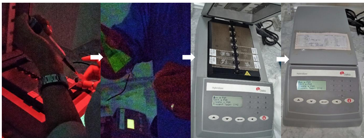
Fig.24. Denaturation of mRNA and hybridization of EBV probe in automatic hybridizer (Original photos)
