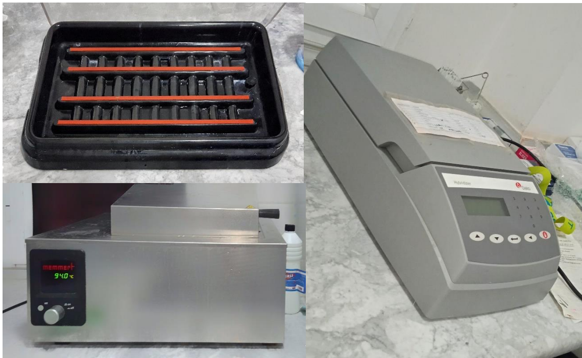
Fig.10 Instruments provided for CISH technique. The right side photo shows the Hybridizer. The up left photo shows the humidity chamber. The low left photo shows the water bath. (Original photos)
