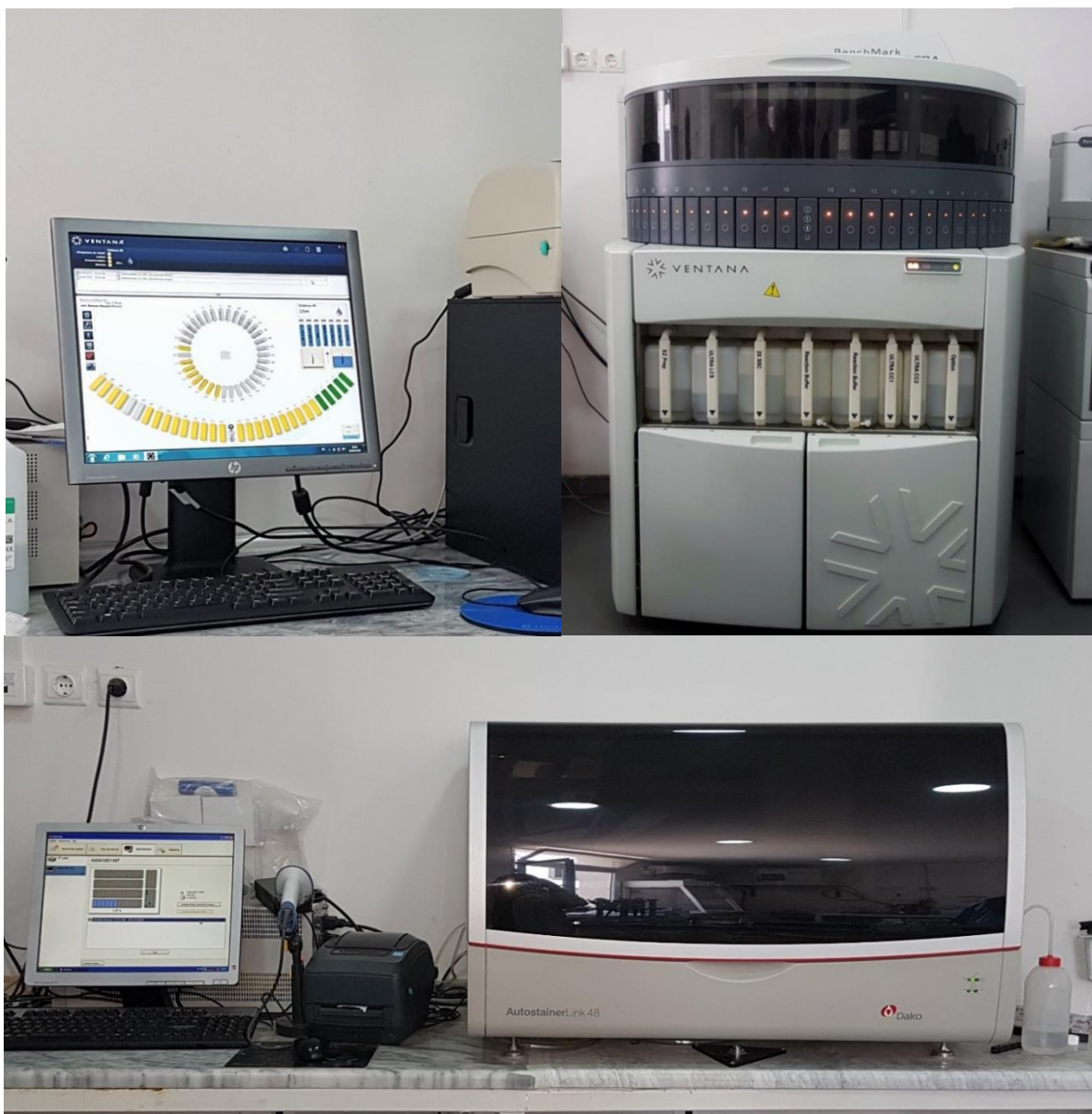
Fig.07 Utilized Autostainers for routine Immunohistochemistry. The upper photo shows the VENTANA BenchMark ULTRA system with the associated software. The lower photo shows the Dako AutostainerLink 48 with the associated software. (Original photos)
