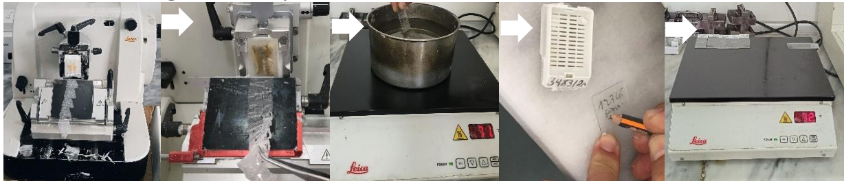
Fig. 15 Histological sections of 1 to 3 \mu m are made with the microtome; the section is spread out on a slide which is then identified and dried on a hot plate. (Original photos)
