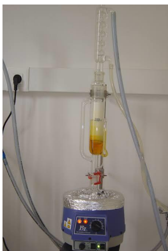
III.7. Extraction soxhlet
