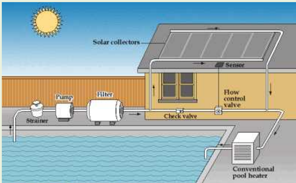
Example of a solar pool heating system.
